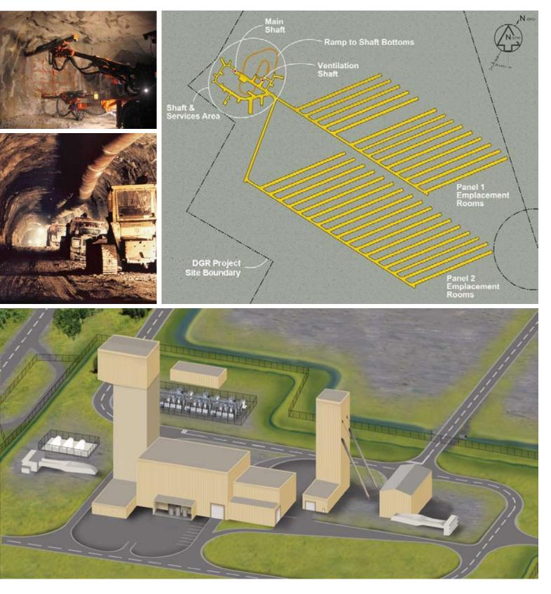
Left top: An example of a drill jumbo creating underground openings in rock
